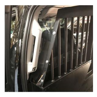
Install Rear Poly Wings at this time using 2ea. 3/4" x 1/4" Hex bolts with flat washers at the predrill locations. You will need to be in the cargo area to install bolts.
