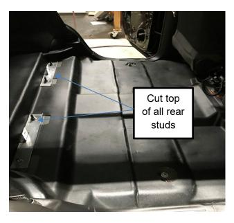
Now you are ready to install the pan. You will need 2 ea. 3/4" x 1/4' bolts, 4 ea. flat washers, and 2 ea. locknuts. These will attach the rear of the pan to the mounting bracket.
