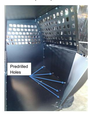
The back must be installed before the front. The back will be very difficult to install if the front is already installed.
