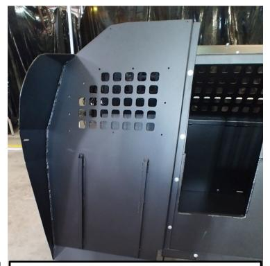
Use 2 ea. ¼" bolts and locknuts in the top through the predrill holes. Use 2 ea. ¼" x bolts and in the bottom section into the predrill holes and nutserts.
