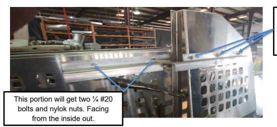
The three nutserted holes will lineup with the top three holes the poly is bolted through.
