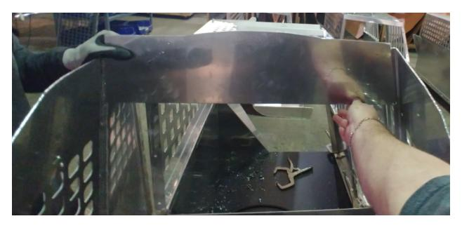
The spit guard will attach with the same bolts that the top of the poly cover and lid connect with. You will need to drill the holes to match in the spit guard. These are the 3 bolts that were left out earlier.
