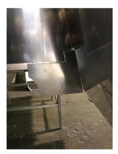
The kick plate will attach with the front bolt that the K9 side piece uses. In the front you will need to drill one more hole and attach.
