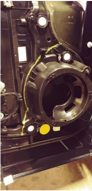
NOTE: It's recommended to use a die grinder with a cut off wheel to remove the speaker pod.
