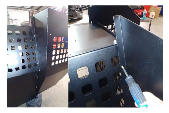
Use 4 ea. bolts and nuts 4 ea. to install the prisoner side back. The prisoner side of the unit is designed to be a tight fit. It may be helpful to utilize an alignment tool to help with getting the holes aligned when installing the bolts.
