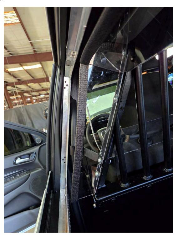
Install Rear Poly Wings at this time. Using 5  $\frac{1}{4}$  20 bolts and flat washers in the nut certed locations
