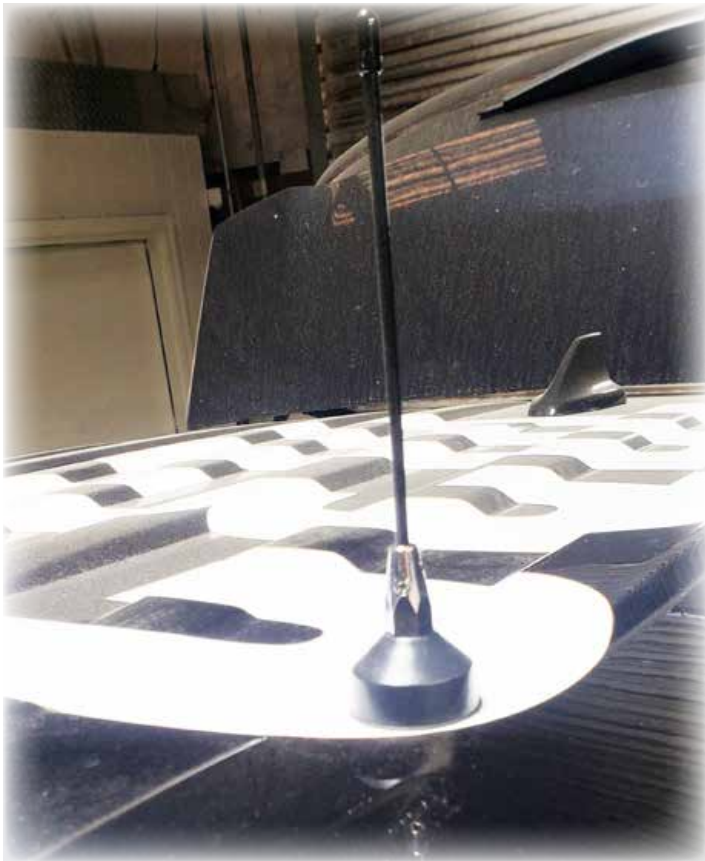
Antenna shown mounted on a Ford Explorer Police Interceptor
