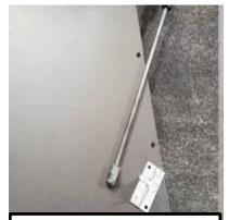
Rivet the bracket onto the front panel with the ball stud facing inward.
