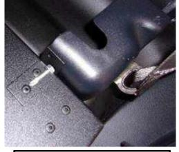
Then take a rubber mallet or a dead blow hammer and tap the tabs into place as shown in picture.
