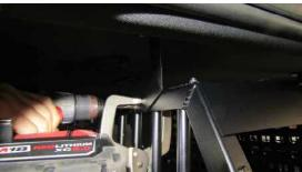
Clamp the bracket to the front angle and drill through making sure to go between the vertical bars.
