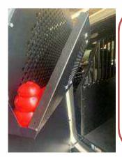
On full platform units a (Fan Guard Shelf) will be mounted on both passenger and driver side window guards. This is a great space that handlers can utilize for storing small light weight items. The downward angle of the (Fan Guard Shelf) also gives a great directional flow of air when equipped with a fan and the K9 is hot and lying prone utilizing a fan.
