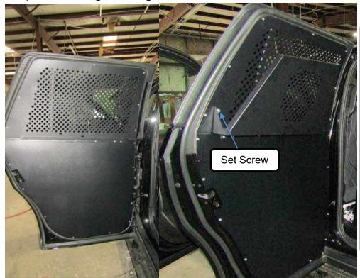
The angled most side of the fan guard shelf will face the latch side of the door and will attach through three corresponding slotted holes on the window guard to allow for proper alignment when installing. Using 3 ea. 1/4" x 5/8" Phillips bolts and lock nuts loosely mount the fan guard shelf and close the door to make sure it does not interact with the K9 cage. Now that the alignment is correct
