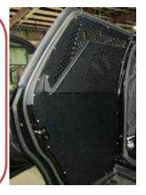
Prior to starting the install the supplied rubber bubble trim should be installed on the bottom of the pan feet and the outside edge of the wings on the back partition.
