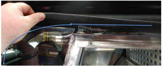
With the trim fully installed you should have a finished look as shown in the photo below.
