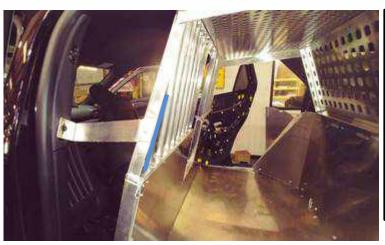
You'll need to remove the factory grab handle. The bracket will be mounted with the factory 10mm grab handle bolt. The rear facing edge of the bracket should line up flush with upper frame of the front. You will then need to drill through the bracket and front. You will then bolt them together 5/8"X 1/4"#20 hex bolt and locking nut.
