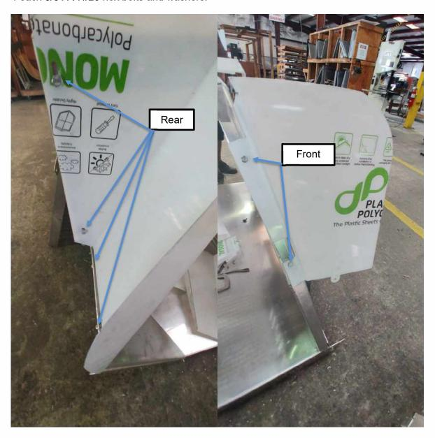
To install the polycarbonate headliner cover you will need to hold the headliner cover in place with the pointed end facing the rear of the vehicle and mark the hole placement. Drill where marked. Attach using 2 each  $5/8 \times 1/4$  #20 hex bolts and washers with lock nuts.
