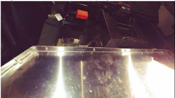
With the vertical slot of the pan bracket and the horizontal slot of the pan lined up place a 5/8" 1/4 #20 bolt with a washer through and attach supplied lock nuts.
