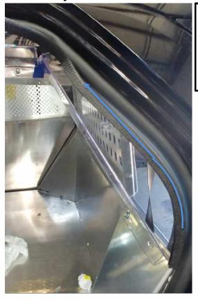
You will need to start installing the trim on the bottom of the rear poly wing. Continuing along the upward edge until the two poly parts come together.
