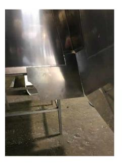
The kick plate will attach with the front bolt that the K9 side piece uses. In the front you will need to drill one more hole and attach.
