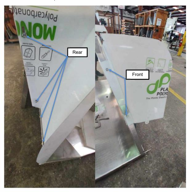
To install the polycarbonate headliner cover you will need to hold the headliner cover in place with the pointed end facing the rear of the vehicle and mark the whole placement. Drill where marked. Attach using 2 each  $5/8 \times 1/4 = 20$  Phillips bolts and washers with lock nuts.
