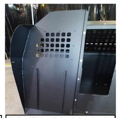
Use 2 ea.  $\frac{1}{4}$ " bolts and locknuts in the top through the predrill holes. Use 2 ea.  $\frac{1}{4}$ " x bolts and in the bottom section into the predrill holes and nutserts.
