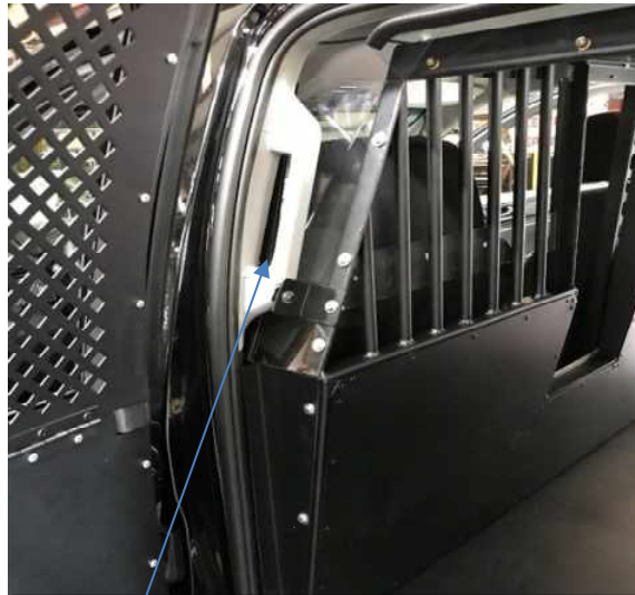
3" tube will go in void behind the tab to give something to tighten against
