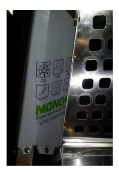
Also you will need to install the Poly between the top of the unit and the door. Using 3 ea. 3/4" x 1/4" bolts with washers per side using the predrilled holes. See detail below.
