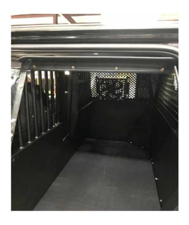
**Step #8 Installing the Rubber Mat**Lay the rubber mat on top of the Pan.
