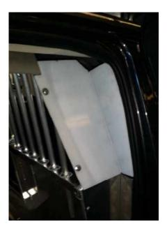
Install Rear Poly Wings at this time. Using  $\frac{1}{4}$  20 hex bolts and flat washers in the nut certed locations
